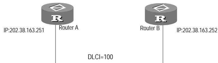
Figure 77 Interconnect LANs via an Annex G DLCI
